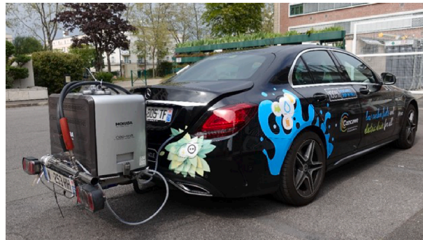
Fig. 4. Vehicle setup for on-road tests, with PEMS equipment.
